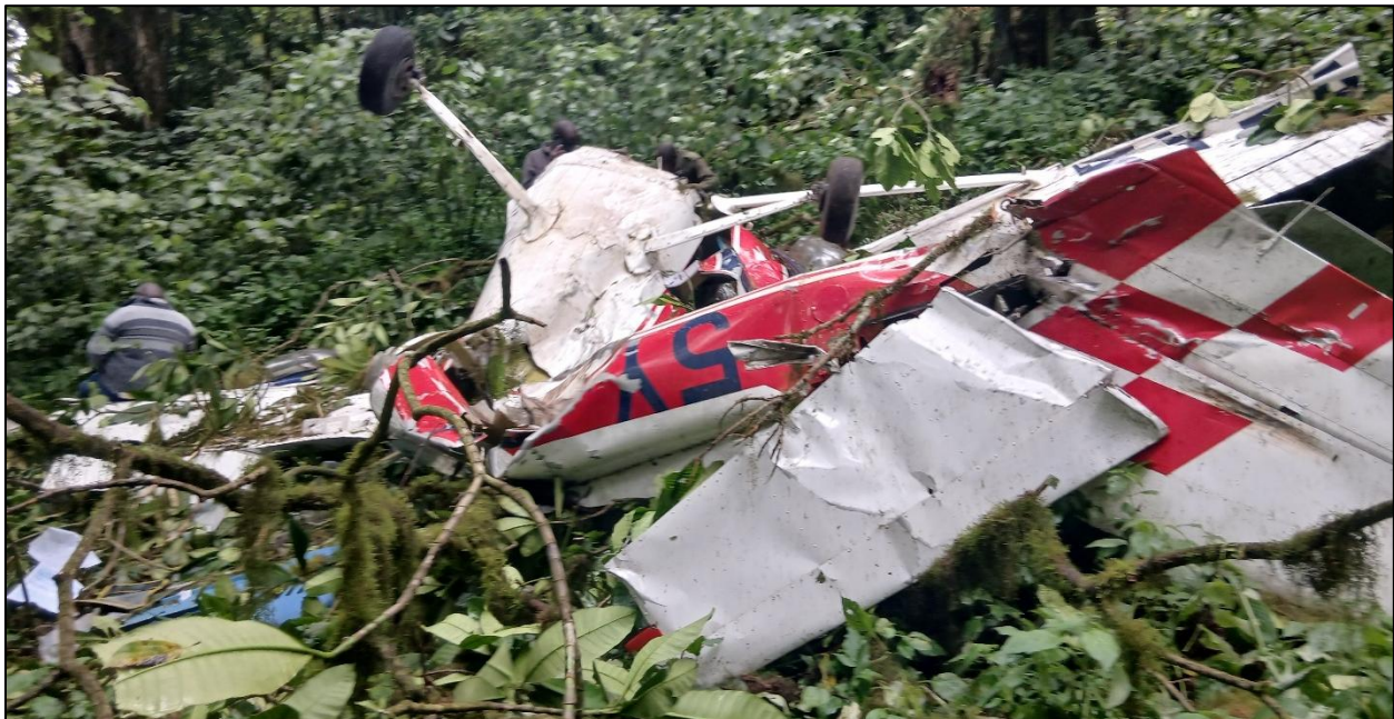
Fig. 4: Photograph showing the extent of damage to the aircraft after impact
