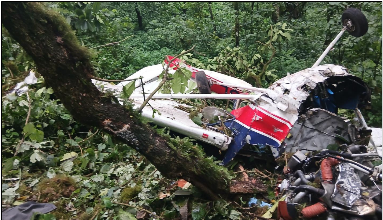
Fig. 3: Photograph showing a tree that broke off and came down with the aircraft on impact
