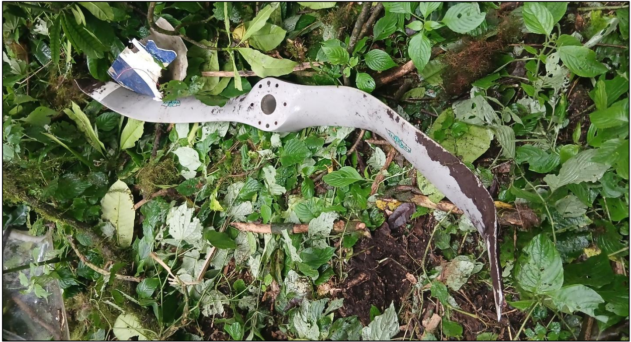
Fig. 5: Photograph showing the propeller blade that separated on impact with the trees
