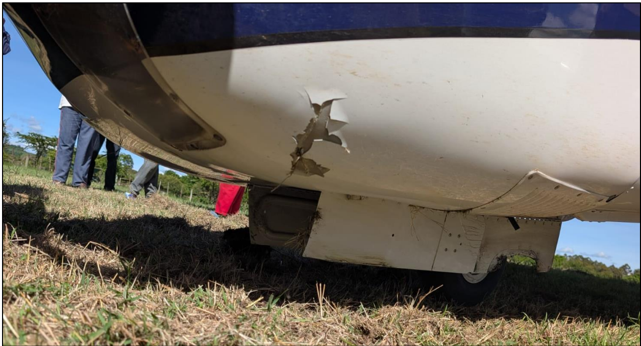
Fig. No. 10: Side view of nose gear damage and lower engine cowling skin delamination.
