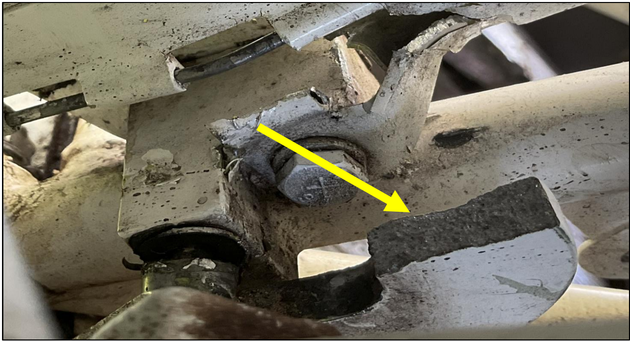
Fig. No. 13: Close-up view of the nose gear down-lock fracture.
