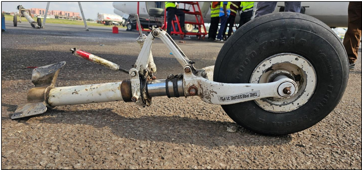
Fig. 6: Photo showing 5Y-BXQ damaged nose gear
