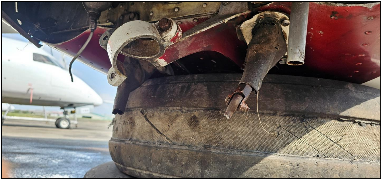
Fig. 4: Photo showing 5Y-BXQ damaged struts and steering tubes
