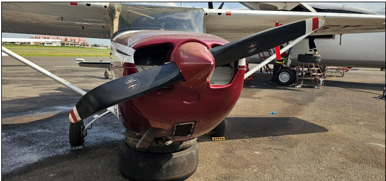
Fig. 3: Photo showing 5Y-BXQ damaged propeller blades
