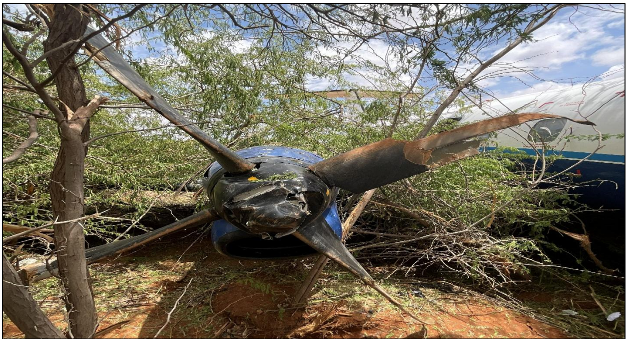
Fig. No. 20: View of Engine No. 2 propeller blades exhibiting mid-span separation and spinner damage
