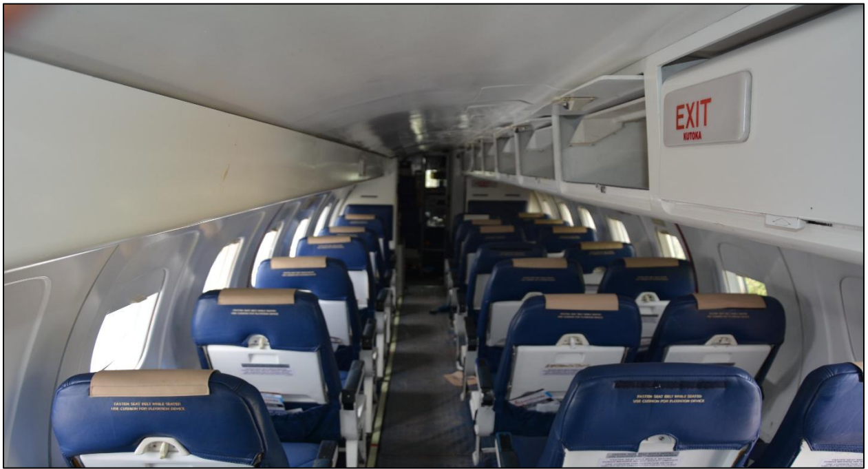
Fig. No. 28: Post-crash cabin interior exhibiting no seat displacement
