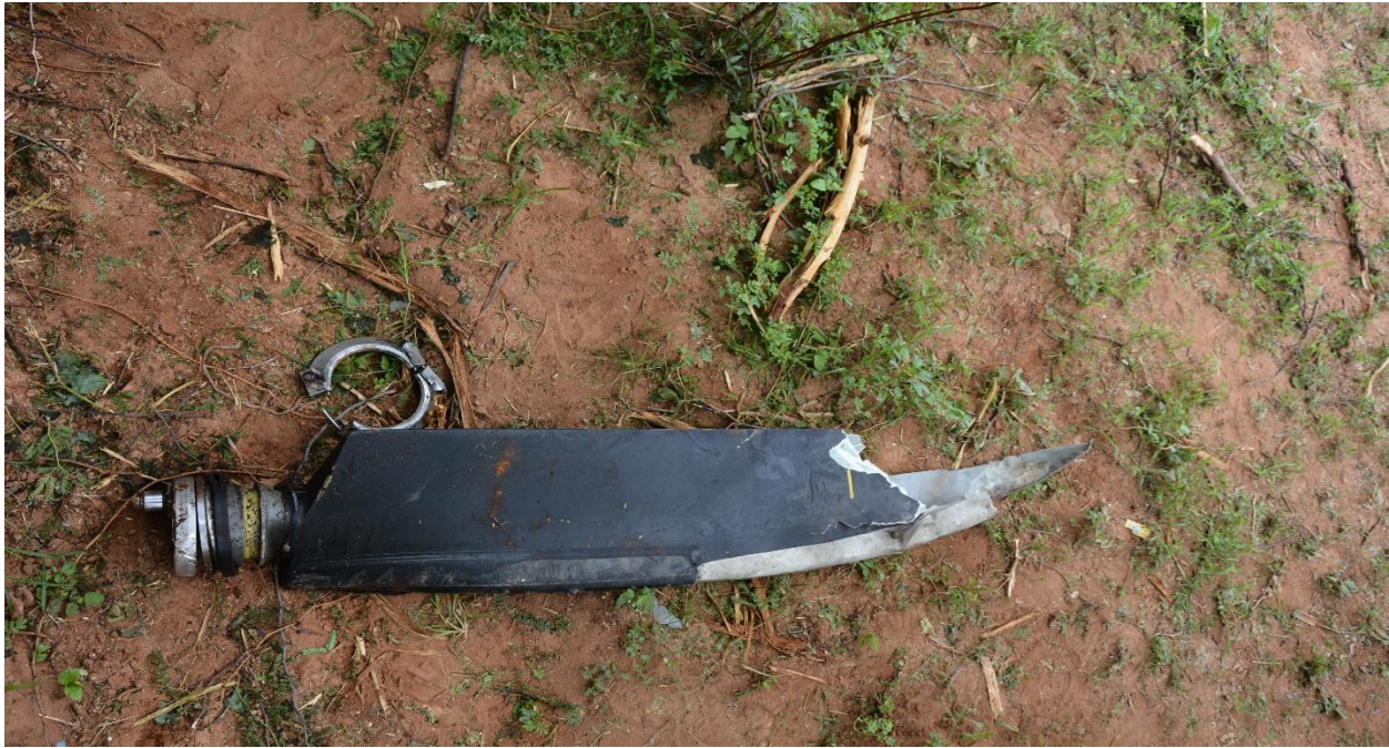
Fig. No. 23: A propeller blade exhibiting torsional damage.
