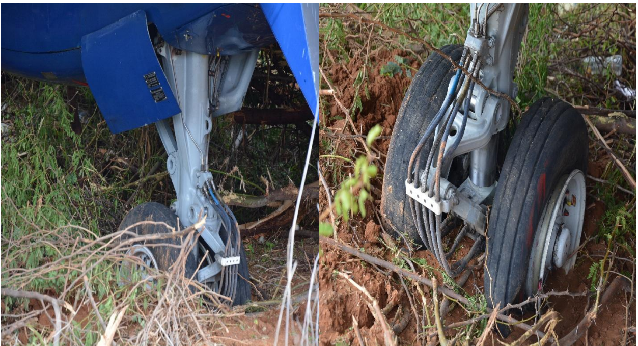
Fig. No. 18: Right main landing gear embedded in the soft ground, and left inboard deflated tire.
