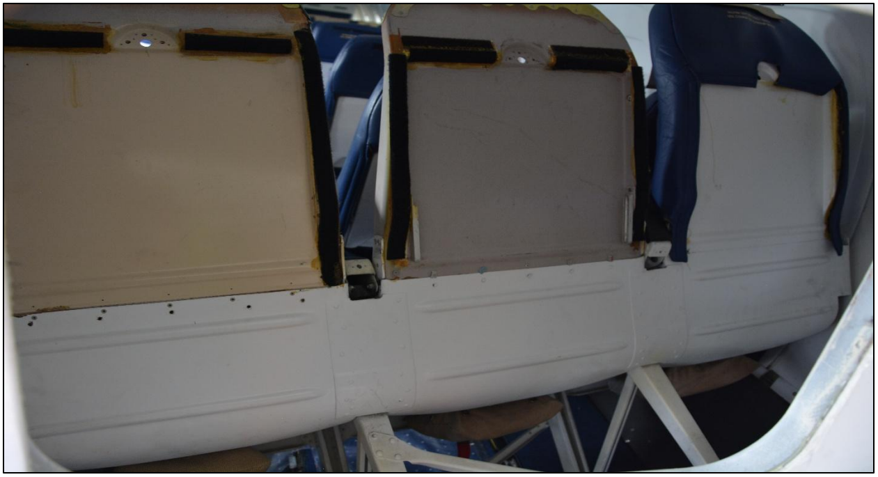
Fig. No. 25: Post-crash aft-row passenger seats and baggage compartment bulkhead/partition exhibiting displacement
