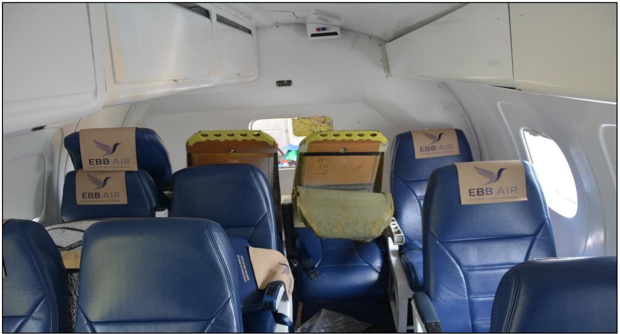
Fig. No. 26: Post-crash aft-row passenger seats and baggage compartment bulkhead/partition exhibiting displacement.
