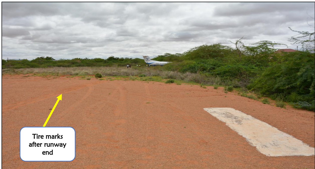
Fig. No. 2: A photo illustrating the runway threshold, tire marks, and the aircraft's final resting position.
