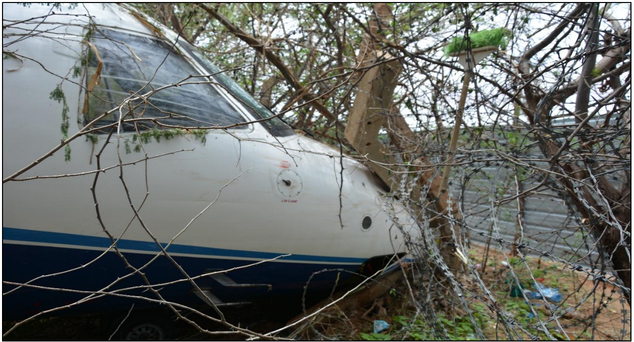
Fig. No. 15: Aircraft entangled in the perimeter fence and associated poles.
