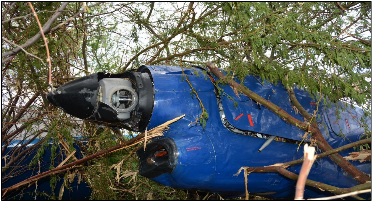
Fig. No. 19: Engine No. 1 propeller hub assembly missing all blades.
