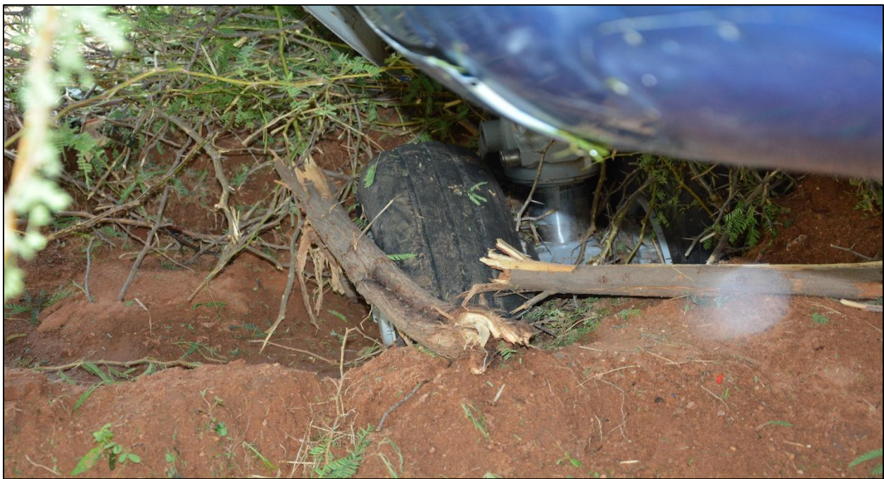
Fig. No. 22: Right main landing gear embedded in the soft ground
