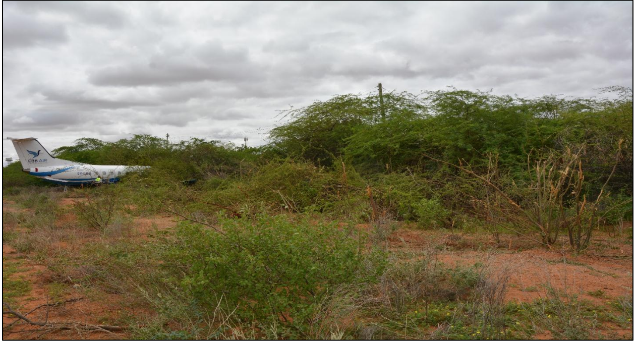
Fig. No. 3: A photo showing the damage to the thicket along the aircraft's direction of motion
