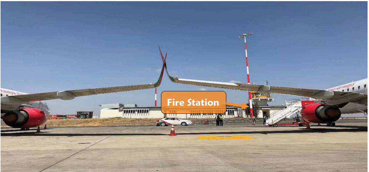
Figure 5: A photo depicting the point of contact of the two aircraft and the fire station in the background.
